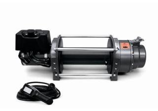
The Series 15 DC features an extended run time high powered DC motor with a weatherproof industrial contactor and heavy duty remote control. The disc brake is designed for extended power-out use. Designed to meet SAE J706 and CE standards. The motor is protected by a thermal overload switch.
