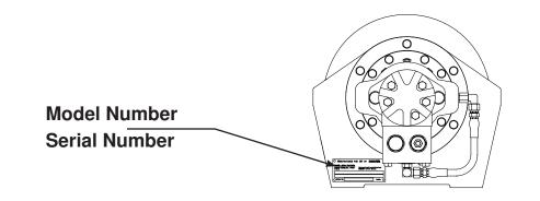
The BRADEN BG6B winch has the model and serial numbers stamped into the brake cylinder endplate. *Always* reference both of these numbers when ordering replacement parts. Our goal is to ship the correct parts, the first time.
