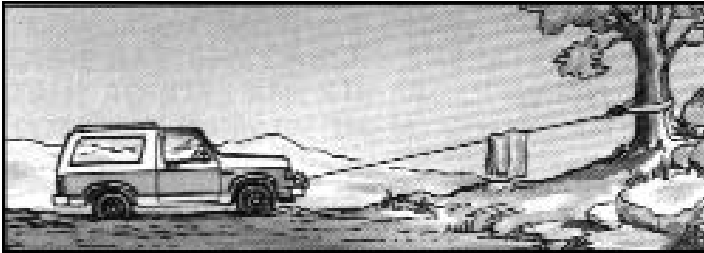
For basic self recovery, anchor to a tree or heavy rock. When anchoring to a tree, always use a tree trunk protector.
