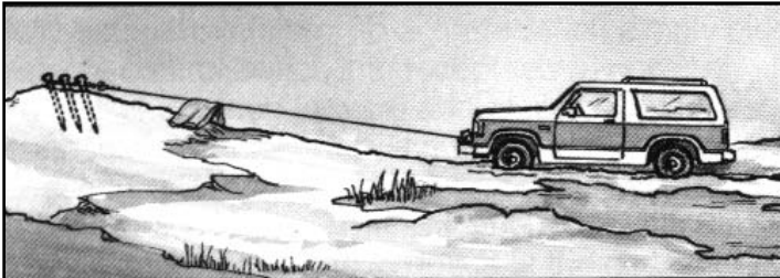
Stakes driven in solid earth and chained together make a good anchor point for self-recovery when no solid anchor point is available.
