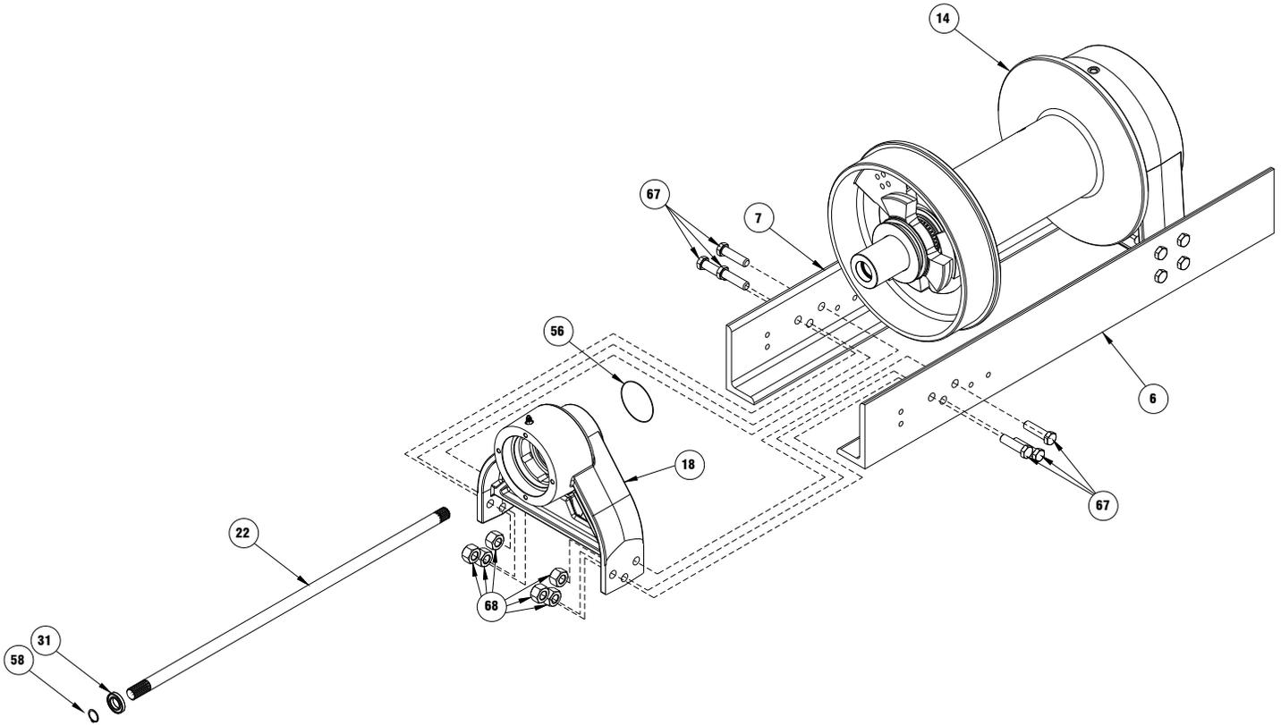
24. While continuing to support the drum #14, remove the clutch #9, snap ring #60 and spacer #25.
