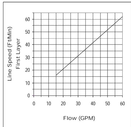
**BASED ON 7.7 CU IN/REV MOTOR**
