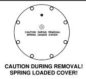
These brakes require no regular adjustment. The direction of braking for all multiple disc brakes can be changed by removing the cam clutch, turning it over, and re-installing it. For detailed service instructions, contact your Tulsa Winch distributor or the factory.
