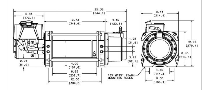
Motor / Contactor may be rotated in 90 degree increments. Clutch housing may be rotated in 72 degree increments.
