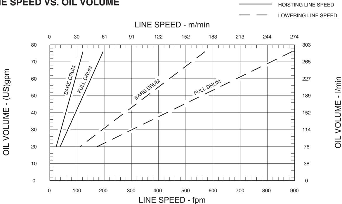
Performance graphs are based on standard hydraulic motor, gear ratio and cable drum with 3/4 inch diameter wire rope.
