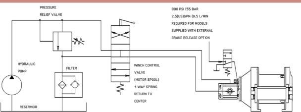
**TYPICAL HYDRAULIC CIRCUIT - STANDARD CONTROL VALUE -** Refer to above hydraulic circuit for installations where the winch is controlled by an individual control valve. Note that the valve must have a motor spool (both winch ports open to tank in neutral position). A motor drain line is not required. Refer to installation manual for alternate circuits.
