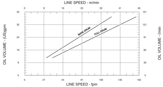
Performance graphs are based on standard hydraulic motor, gear ratio and cable drum with 1/2 inch diameter wire rope.
