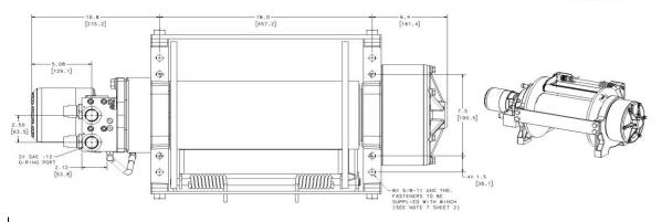
Motor / Contactor may be rotated in 90 degree increments. Clutch housing may be rotated in 60 degree increments.
